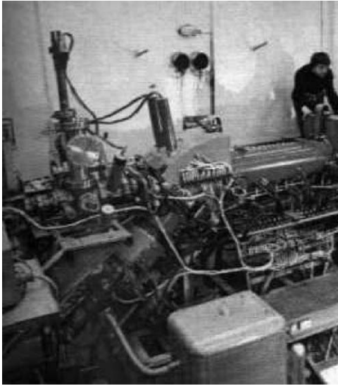
Fig. 1. The beginning of Electron Cooling Epoch: the first electron cooler EPOkhA at Budker INP, Novosibirsk (Rus. Abbreviation “Electron Beam to Cool Antiprotons”).
