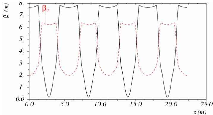
**FIGURE 1.** USR lattice functions at the working point  $Q_x=2.29$ ,  $Q_y=1.08$  as calculated with MAD.
