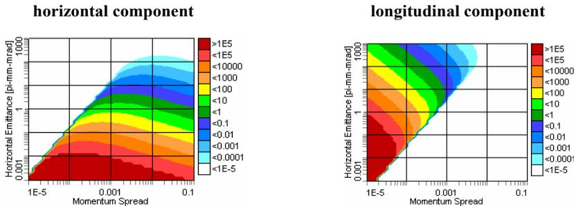
**FIGURE 2.** Intra-beam scattering heating rates (positive).
