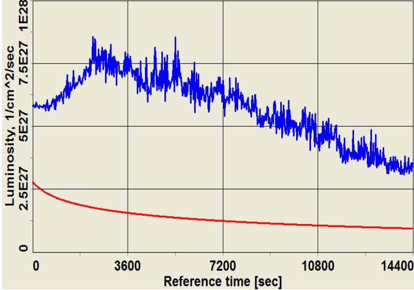
**FIGURE 1.** Luminosity of RHIC for gold-gold collisions at 100 GeV/A per beam as a function of time in collision with magnetized cooling. The red line represents the luminosity without electron cooling, which decays due to IBS. The blue curve represents the luminosity of the cooled collider. The decline in luminosity here is due to ion beam loss by disintegration in the interaction points.
