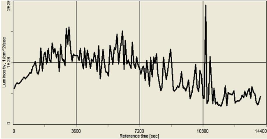
**FIGURE 4.** Luminosity of RHIC for gold-gold collisions at 100 GeV/A per beam as a function of time in collision with non-magnetized cooling. The decline in luminosity here is due to ion beam loss by disintegration in the interaction points in combination with recombination losses. The spikes are artifacts of the simulation.
