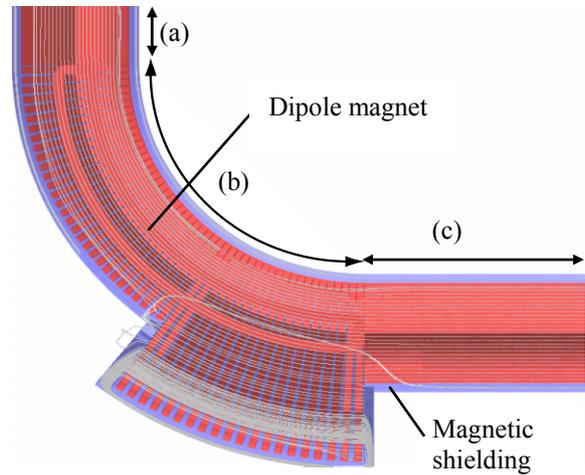
Figure 4: Flux lines started from the mid-plane of the cooling solenoid and the large diameter solenoids. The notations of (a), (b), and (c) are indicated in the figure 3.
