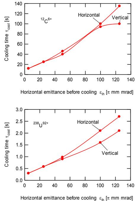
Figure 1: The dependence of cooling time on the horizontal emittance for (a)  $^{12}\text{C}^{6+}$ , 400 MeV/u,  $I_e = 4$  A, and (b)  $^{238}\text{U}^{92+}$ , 100 MeV/u,  $I_e = 1$  A. The initial ion beam has the parameters of  $\delta p/p = 0.00015$ ,  $\epsilon_v = 40 \pi$  mm mrad, and the electron cooler  $T_{e\perp} = 5$  meV,  $B_{\text{gun}} = 4$  kG,  $B_{\text{cool}} = 2$  kG.
