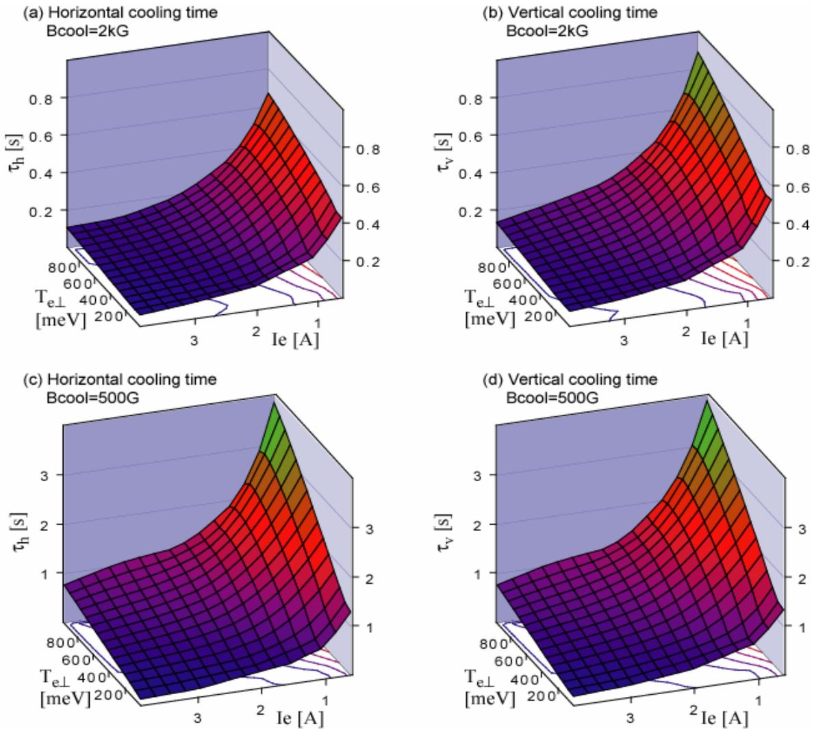
Figure 2: The dependence of horizontal and vertical cooling time for  $^{238}\text{U}^{92+}$  on the transverse electron temperature and the electron beam current. The magnetic field in the cooling section was applied to 2 kG for (a) and (b), and 500 G for (c) and (d), respectively.
