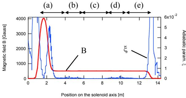
Figure 3: Magnetic field and adiabatic parameters on the solenoid axis; (a) gun section, (b) toroidal section, (c) cooling section, (d) toroidal section, and (e) collector section, respectively.
