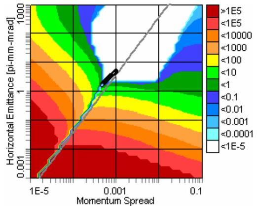
Figure 6: Result from overlapping the before-mentioned rates and the effects of the rest gas. Dynamics during the cooling process is given by the black points in the figure.
