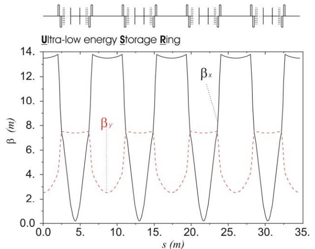
Figure 1: Betafunctions of the USR as calculated with the MAD code.  $Q_x=2.38$ ,  $Q_y=1.14$ .
