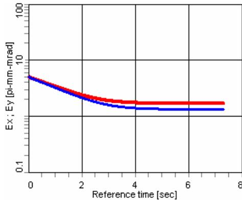
Figure 7: Evolution of the horizontal and vertical emittance during the cooling process.
