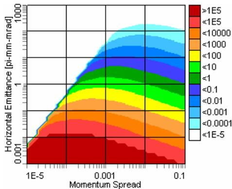
Figure 2: Transverse IBS heating rates (positive).
