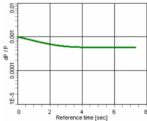
Figure 8: Momentum spread of the stored beam as a function of time during the cooling process.
