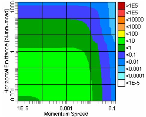
Figure 4: Electron cooling rates (negative) of the transverse component.
