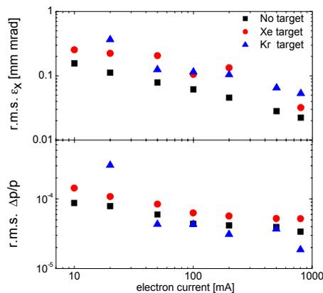
Figure 3: Equilibrium beam parameters versus the electron current in the cooler for Kr and Xe targets. No equilibrium was reached with Kr target for  $I_e < 20$  mA.
