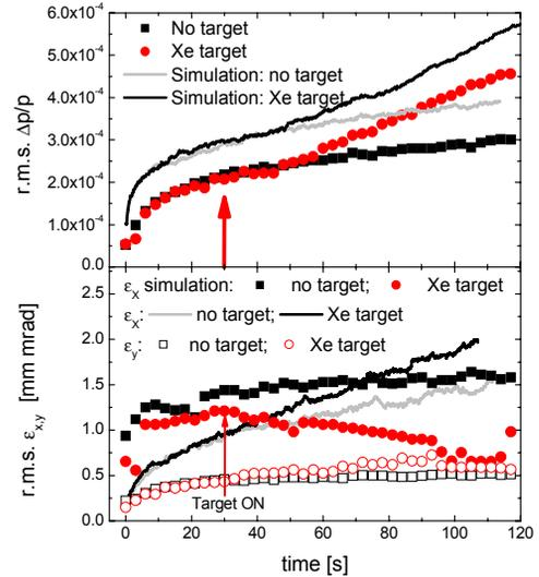
Figure 2: Evolution of  $\Delta p/p$  and  $\epsilon_{x,y}$  for Xe target ( $2.5 \times 10^{12}$  atoms/cm<sup>2</sup>) compared with BETACOOL result for an 'effective' density of  $6.2 \times 10^{11}$  atoms/cm<sup>2</sup>.
