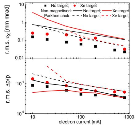
Figure 4: Same as in Fig. 3 for Xe target, compared with BETACOOOL simulations using non-magnetised and Parkhomchuk electron cooling model.
