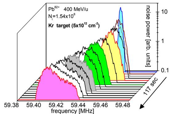
Figure 1: Longitudinal Schottky spectra recorded every 9 s during the blow-up measurement with the cooler OFF. The target is ON at  $t \approx 30 \text{ s}$ . Different colors are used to guide the eye.
