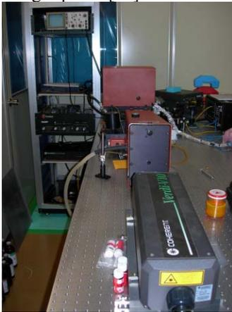
Figure 6: Ring dye laser followed by a second harmonics generator tuned to the average power level of -30mW.
