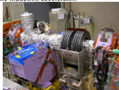
Figure 5: Untuned RF cavity with upper cover removed and the induction accelerator with upper part removed
