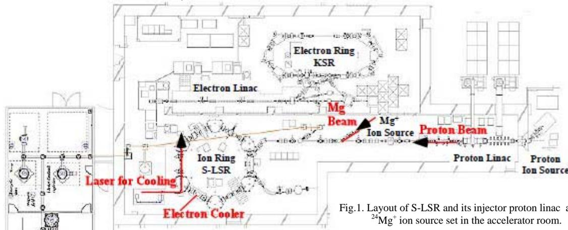
Fig.1. Layout of S-LSR and its injector proton linac and  $^{24}\text{Mg}^+$  ion source set in the accelerator room.
