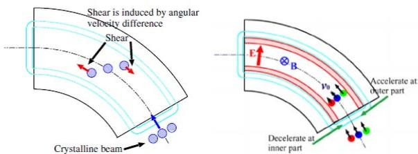
Fig.4 Illustration of shear [15]. Fig. 5 Dispersion suppressor using a cross electric field with a magnetic field [15].
