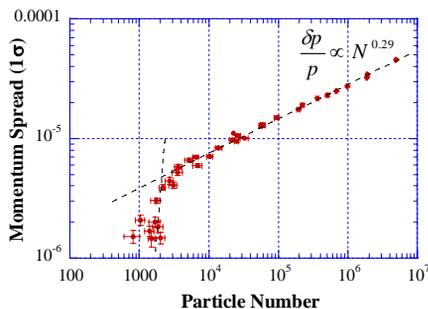
Fig. 2. Observed abrupt jump of momentum spread of 7 MeV proton beam at particle number  $\sim 2000$ , which is considered to be the evidence of the phase transition to 1 dimensional ordered state [11].
