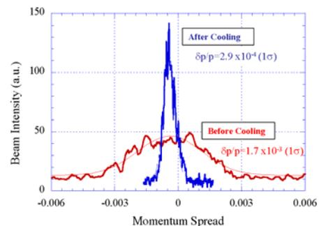
Fig. 3 Result of laser cooling on  $^{24}\text{Mg}^+$  ions. Laser cooling was applied to  $\sim 10^8$   $^{24}\text{Mg}^+$  ions together with an induction deceleration voltage of  $\sim 6$  mV, which reduced the fractional momentum spread from  $1.7 \times 10^{-3}$  to  $2.9 \times 10^{-4}$ . The spectrum after cooling was measured 5 second after the start of laser cooling.
