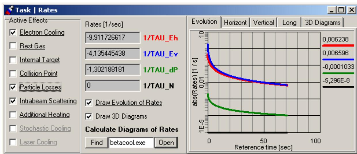
Figure 1: Form for the control of active effects and visualisation of growth rate evolution
