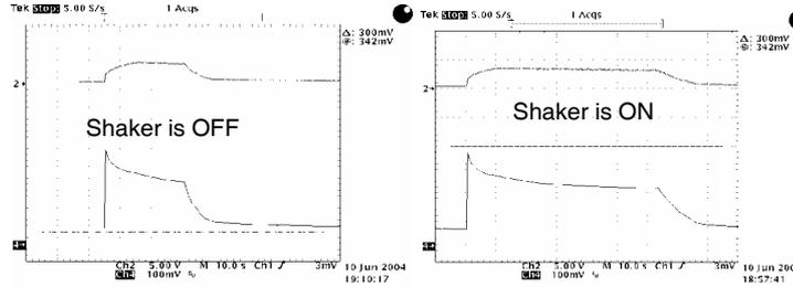
Figure 3: The shaker effect. Upper curves –  $H^0(t)$ , lower curves –  $I_p(t)$ .
