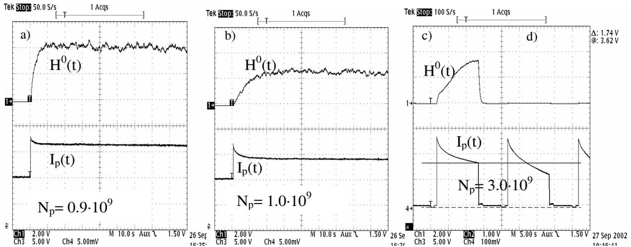
Figure 1: Dependence of neutral hydrogen flux  $H^0(t)$  and proton beam current  $I_p(t)$  on time at single injection shot in COSY at different injected proton number  $N_p$  and beam emittance values:  $3\epsilon_a \approx \epsilon_b \approx \epsilon_c$  when electron cooling is ON (a, b, c) and OFF (d,  $H^0(t) \equiv 0$ ).
