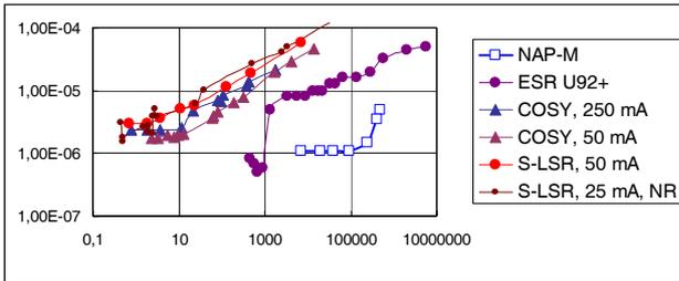
Figure 4: Comparison of the beam ordering experiments at NAP-M, ESR, COSY and S-LSR: particle momentum spread vs the “ordering parameter”.
