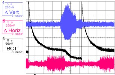
Figure 2: Rare repetition of injection at COSY (two shots are shown): proton beam (a) and signals of vertical (b) and horizontal (c) PU-monitors vs time (5 s/div).
