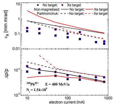
Figure 2: Equilibrium horizontal emittance and momentum spread (r.m.s. values) versus electron current of the cooler for Xe target ( $2.5 \times 10^{12}$  atoms/cm<sup>2</sup>).
