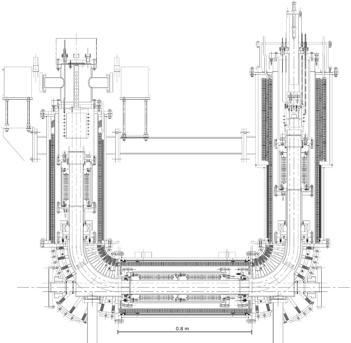
Fig. 1. A cross-sectional view of the S-LSR electron cooler. The toroid of radius 0.25 m has 9 discrete coils. The straight section is 0.8 m in length. The magnetic field in the cooling section is 500 G and the maximum expansion factor is 3
