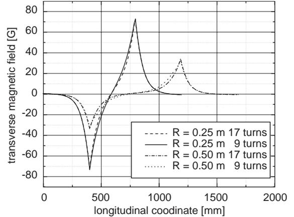
Fig. 3. Dependence of the transverse field on the bending radius of the toroidal section.
