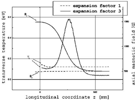
Fig. 2. Reduction of the transverse electron beam temperature by adiabatic expansion ( $I_e = 300$  mA).
