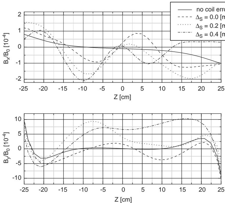
Fig. 4. Dependence of transverse field distributions on the systematic coil errors ( $B_0 = 500$  G).
