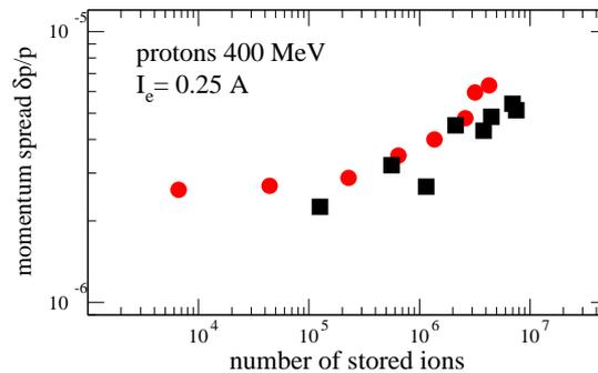
Figure 2: Measurement of the momentum spread ( $2\sigma$ ) of a proton beam at 400 MeV cooled with an electron current of 250 mA. By connecting a resonant circuit to the Schottky pick-up (red circles) the sensitivity could be increased by more than one order of magnitude.
