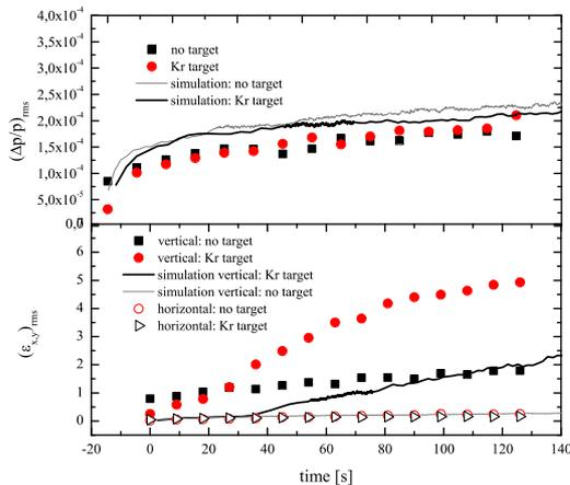
Figure 1: Comparison of measurement and BETACOOOL simulation of the longitudinal and transverse heating of a bare nickel beam at 400 MeV/u interacting with a Kr target of  $6 \times 10^{12}$  atoms/cm<sup>2</sup>. The initial heating is due to intrabeam scattering, the target is switched on after 30 s.
