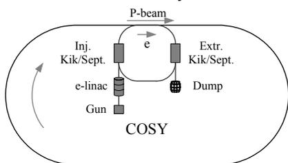
Fig. 1: Layout of a linac-based MEEC system
