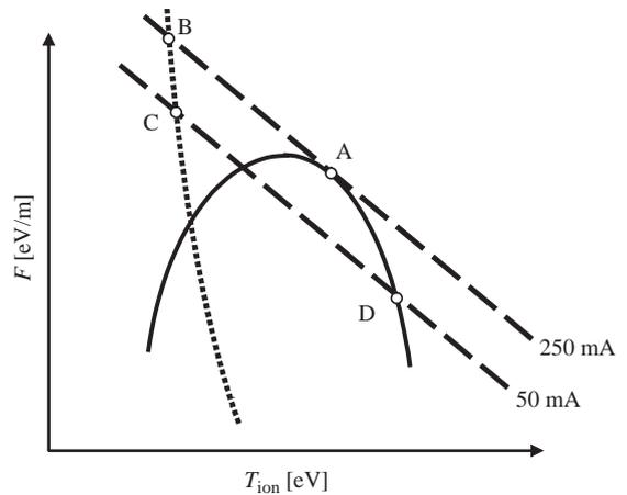
Fig. 2. The dependence of cooling and heating forces on the ion temperature. Solid line corresponds to IBS, dashed line—to ECOOL with negative sign, dotted line—to other heating process.
