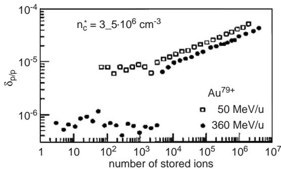
Fig. 1. Momentum spread for different power supply stability of electron cooler. The power supply for energy of 360 MeV/u is more stable than for energy 50 MeV/u (ESR experiment).
