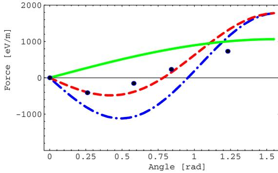
FIG. 7. (Color) Transverse component of the force. Comparison for  $\Delta_{e,\perp} = 4.2 \times 10^5$  m/s: blue dot-dashed line—Eq. (6); red dashed line—Eq. (8); green solid line—Eq. (9); dots with error bars—VORPAL results.
