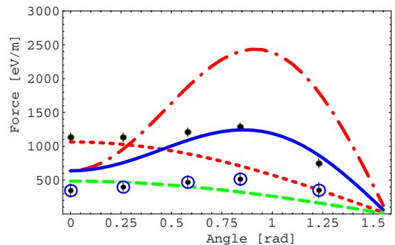
FIG. 4. (Color) Longitudinal component of the force: (1) For  $\Delta_{e,\perp} = 4.2 \times 10^5$  m/s: red (dot-dashed) line—Eq. (5); red short-dashed line—Eq. (9); dots with error bars—VORPAL results. (2) For  $\Delta_{e,\perp} = 1.1 \times 10^7$  m/s: blue solid line—Eq. (5); green long-dashed line—Eq. (9); open circles with error bars—VORPAL.
