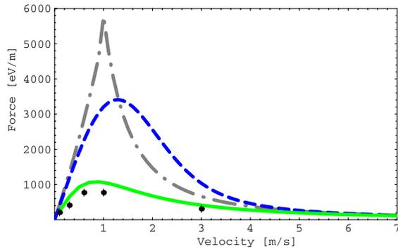
FIG. 2. (Color) Longitudinal component of the force (eV/m) vs ion velocity ( $\times 10^5$  m/s). BETACOOOL results: solid line (green)—Eq. (9); dot-dashed line (gray)—asymptotics [4]; dashed line (blue)—Eq. (4); VORPAL results: dots with error bars.
