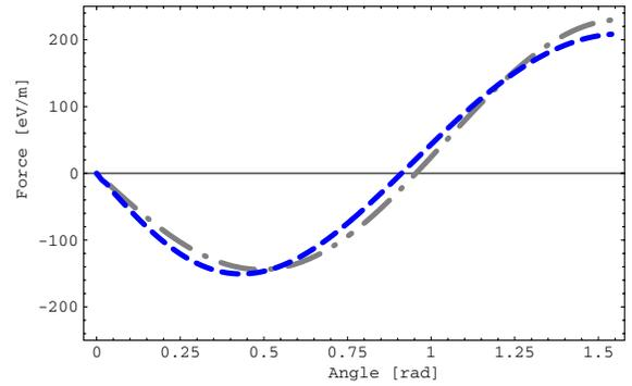
FIG. 9. (Color) Transverse component of the force at ion velocity  $6 \times 10^5$  m/s ( $\Delta_{e,\perp} = 1.1 \times 10^7$  m/s,  $\Delta_{e,\parallel} = 1.0 \times 10^5$  m/s,  $B = 5$  T): gray dot-dashed line—Eq. (6); blue dashed line—Eq. (4).
