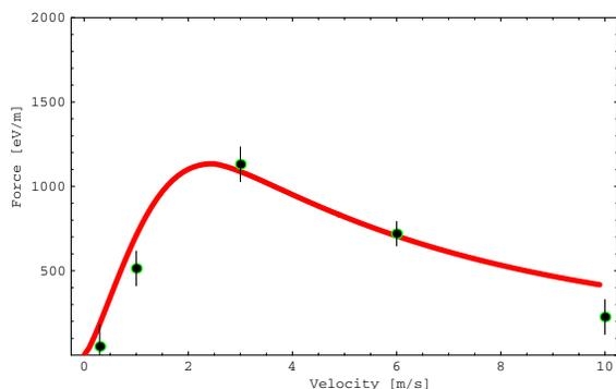
FIG. 1. (Color) Nonmagnetized force (eV/m) vs ion velocity ( $\times 10^5$  m/s) for an anisotropic velocity distribution: solid line—Eq. (3) implemented in BETACOOOL; points with error bars—simulations using VORPAL.
