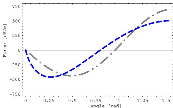
FIG. 8. (Color) Transverse component of the force at ion velocity  $3 \times 10^5$  m/s ( $\Delta_{e,\perp} = 1.1 \times 10^7$  m/s,  $\Delta_{e,\parallel} = 1.0 \times 10^5$  m/s,  $B = 5$  T): gray dot-dashed line—Eq. (6); blue dashed line—Eq. (4).
