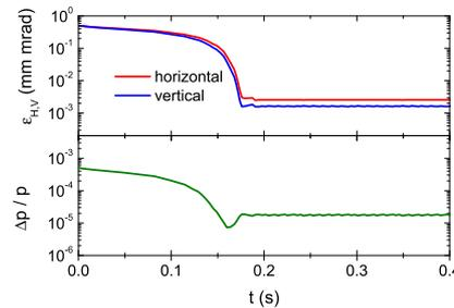
Figure 1: Simulation of electron cooling of a coasting beam of  $10^8$   $^{132}\text{Sn}^{50+}$  ions at 740 MeV/u. The initial beam parameters correspond to the pre-cooled beam from CR. Electron beam current: 1 A.
