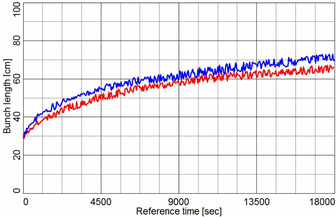
Figure 2: Evolution of RMS bunch length for Au ion bunch with beam parameters in Table 2. Red lower curve – for bunch intensity  $1 \times 10^9$ ; blue upper curve – for bunch intensity  $1.5 \times 10^9$ .
