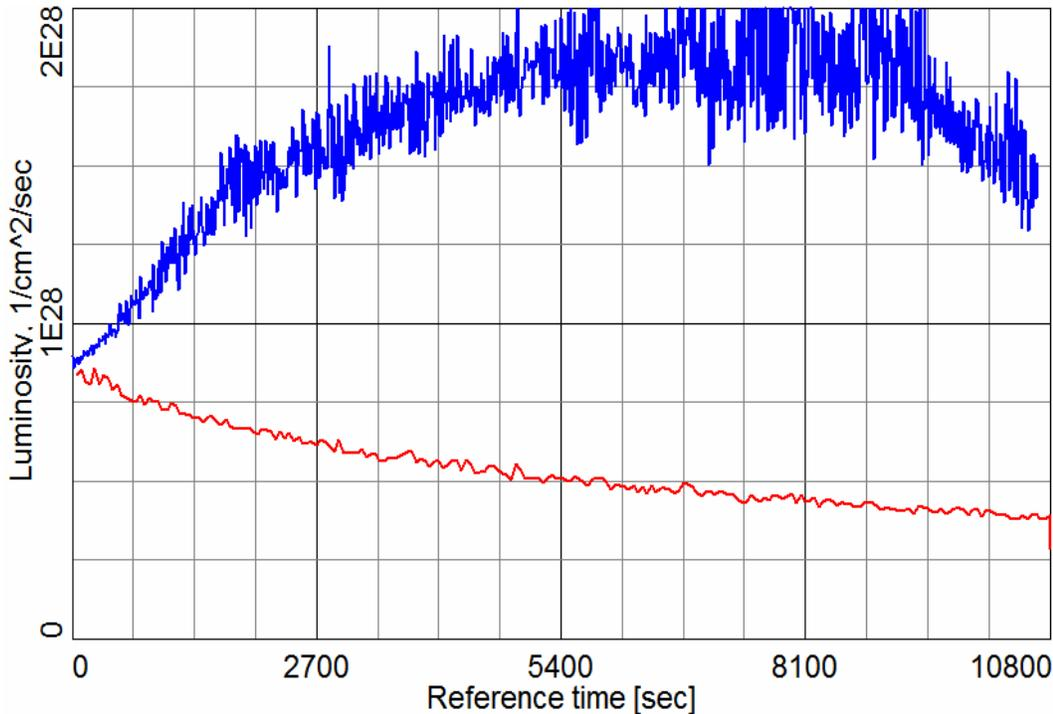
Figure 15. Luminosity of Au ions at 100 GeV/nucleon for ion bunch intensity of  $N_i = 1.5 \cdot 10^9$ ,  $\beta^* = 0.8\text{m}$ : with electron cooling (blue upper curve) and without cooling (red lower curve).
