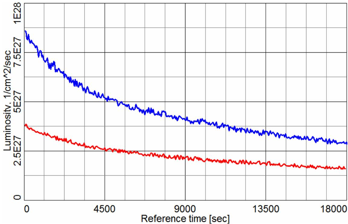
Figure 3: Resulting luminosity for 112 Au ions bunches,  $\beta^*=0.8$  m for beam parameters in Table 2. Red lower curve – for bunch intensity  $1 \times 10^9$ ; blue upper curve – for bunch intensity  $1.5 \times 10^9$ .
