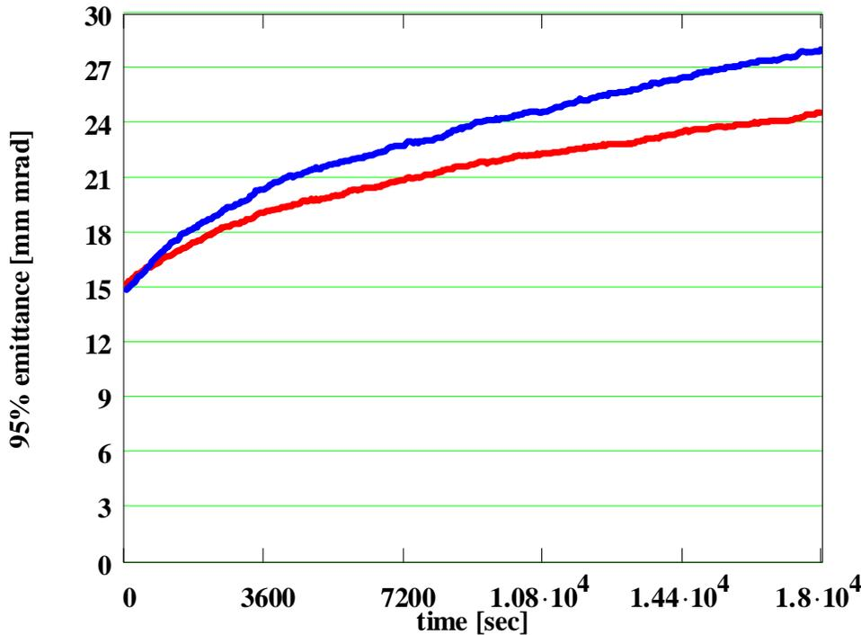
Figure 1: Evolution of 95% normalized transverse emittance for Au ions with beam parameters in Table 2. Red lower curve – for bunch intensity  $1 \times 10^9$ ; blue upper curve – for bunch intensity  $1.5 \times 10^9$  (using IBS-lattice “dAu82” from 2008 RHIC physics run in Yellow ring).
