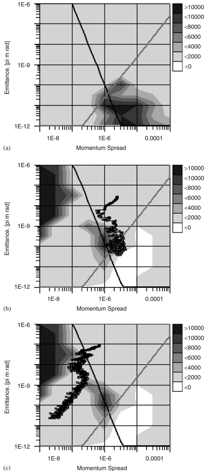
Fig. 4. MD simulation: (a) Horizontal component of IBS growth rates, (b) longitudinal component of IBS and (c) evolution of beam parameters during cooling process.  $I_{cool} = 5$  A,  $^{132}\text{Sn}^{50+}$  220 MeV/u,  $N = 10^5$ .
