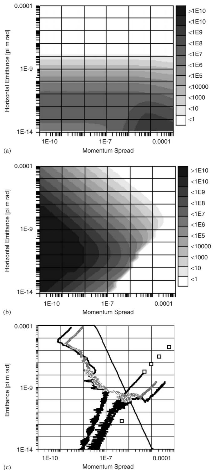
Fig. 3. Theoretical dependence of IBS growth rates on beam emittance and momentum spread for ESR: (a) horizontal and (b) longitudinal components of IBS growth rates. Results of MD calculations (c): evolution of ion beam parameters during cooling. Solid black line corresponds to cooling rate of  $4 \times 10^4$  Hz. Grey circles correspond to cooling rate of  $10^4$  Hz. Straight line is criterion  $\Gamma_2 = \pi$  ( $N = 5 \times 10^5$ ). Open squares are ESR experiment (see Fig. 2).
