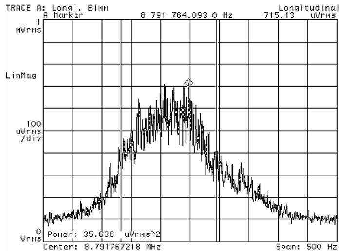
Fig.3.4. Schottky signal for particle number  $10^7$ .
