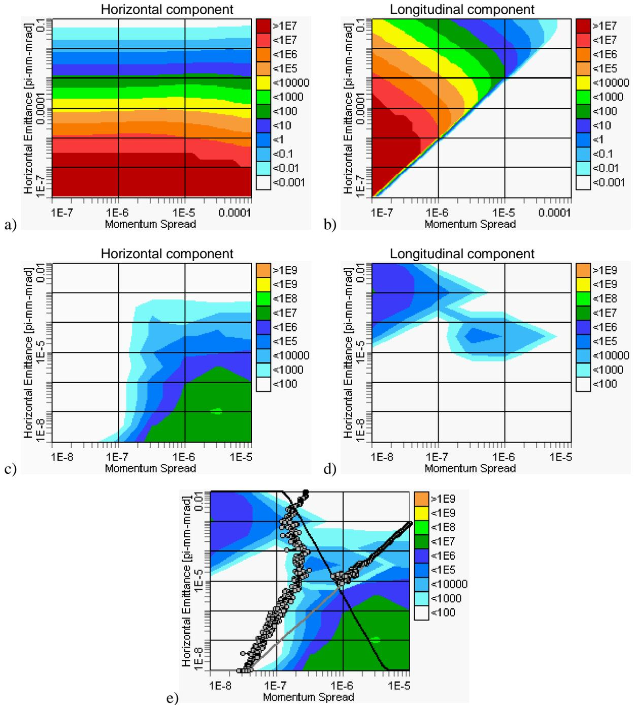
Fig.2.6. Growth rates of IBS and proton beam parameters evolution (gray squares) at electron cooling in COSY,  $N_p = 10^6$ .
