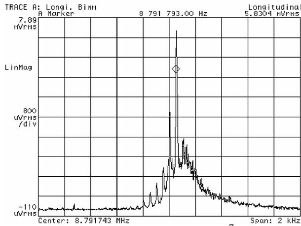
Fig.3.10. Schottky noise spectrum at  $10^7$  proton number (the same as in Fig.3.4) and transverse heating by white noise.
