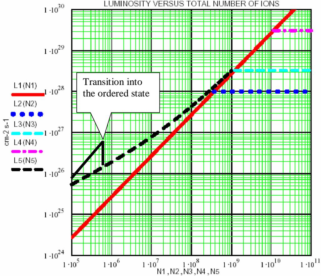
Fig. 1. Luminosity dependence on the ion number. Solid red line corresponds to the constant beam-beam parameter  $\xi_i = 0.045$ . Three upper horizontal lines correspond to a limitation due to the space charge effect for different ion species. Black dashed line shows the luminosity benefit due to higher  $\xi_i$  at decrease of the ion beam emittance. The solid black line – luminosity after transition into the ordered state.
