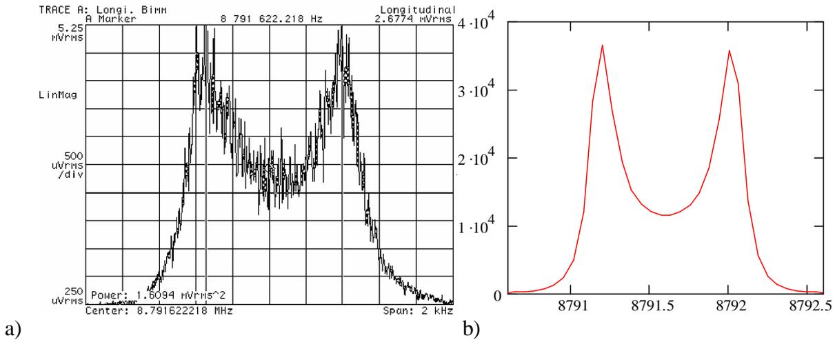
Fig.3.2. Shape of the Schottky spectrum with two peaks. a) signal measured in the experiment, b) fitting curve in accordance with (3.1) - amplitude is in arbitrary units, frequency is in kHz,
