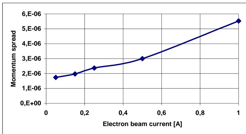
Fig.3.8. The dependence of minimum momentum spread on electron beam current.
