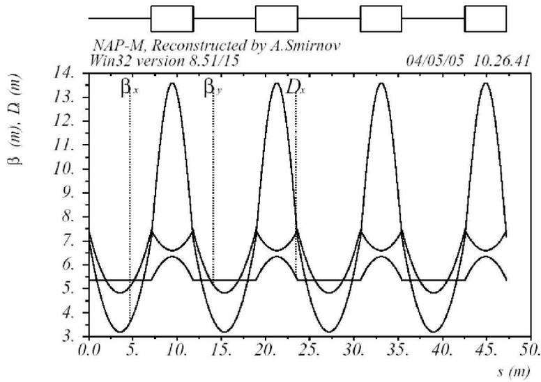
Fig.2.2. Lattice structure of NAP-M.
