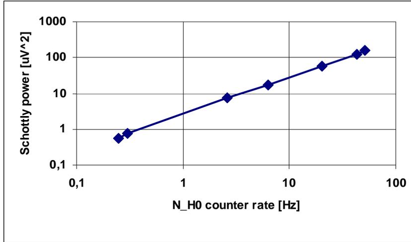
Fig.3.5. Calibration of Schottky signal power with  $H^0$  monitor in COSY.
