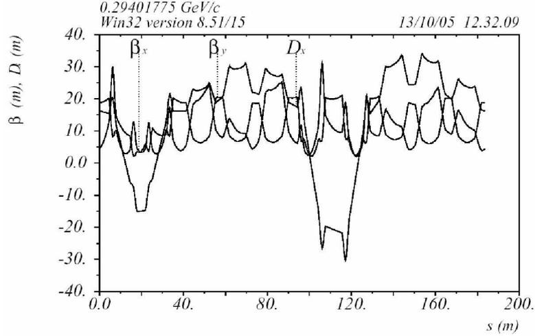
Fig.3.1. COSY Lattice structure at injection energy.
