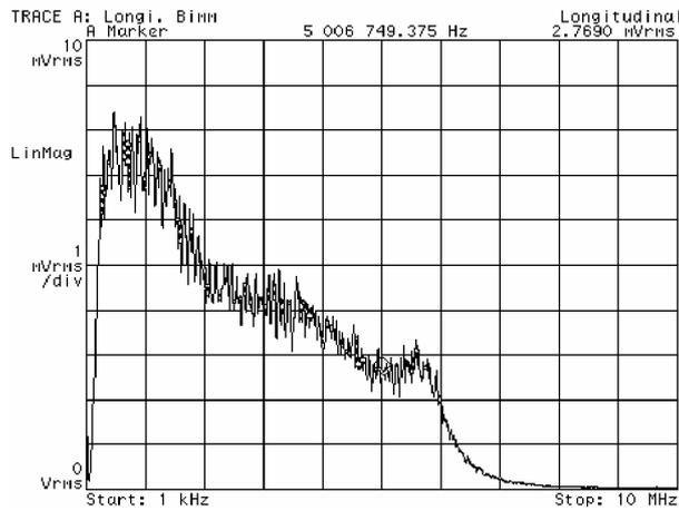
Fig.3.9. Spectrum of the noise signal used for the transverse heating of the proton beam.
