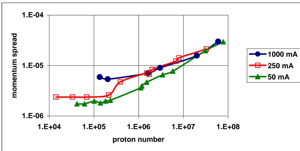
Fig.3.7. The dependence of momentum spread on the proton number for different values of electron beam current
