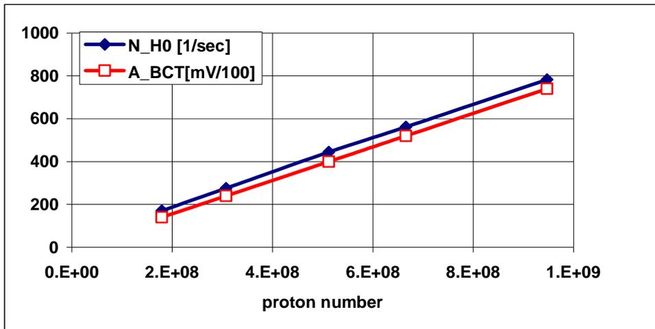
Fig.3.3. Calibration of  $H^0$  monitor with BCT.  $I_e=250$  mA.
