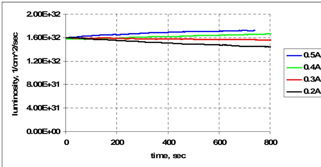
Fig.2.6. The dependence of luminosity for bunched beam on time for different values of electron beam current.
