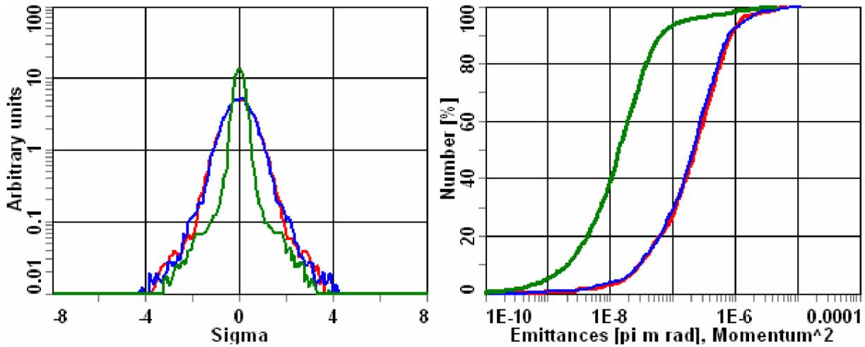
Fig.2.11. Transverse (a, red and blue) and longitudinal (a, green) profiles and sorted invariants (b) of cooled bunched beam ( $I_e = 0.2$  A)
