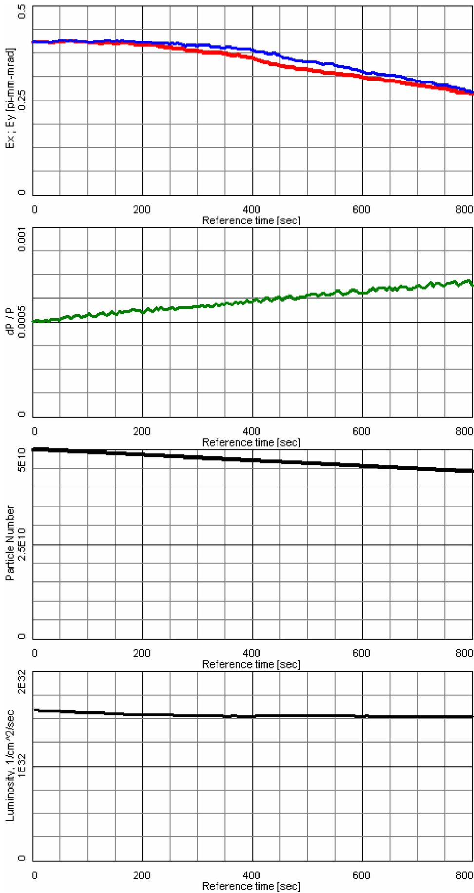
Fig. 3.3. From top to bottom: evolution of the beam emittance, momentum spread, proton number and luminosity under the common action of internal target, intrabeam scattering and transverse stochastic cooling. Initial effective target thickness is  $2 \cdot 10^{15}$  Atoms/cm<sup>2</sup>.
