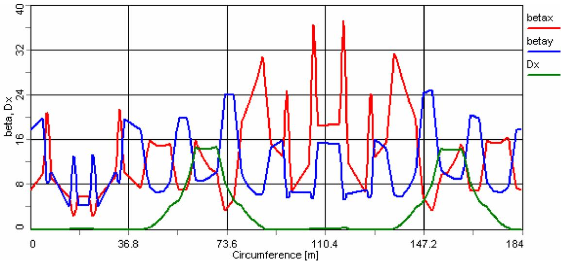
Fig. 2.1. Lattice parameters used in simulation of intrabeam scattering process.
