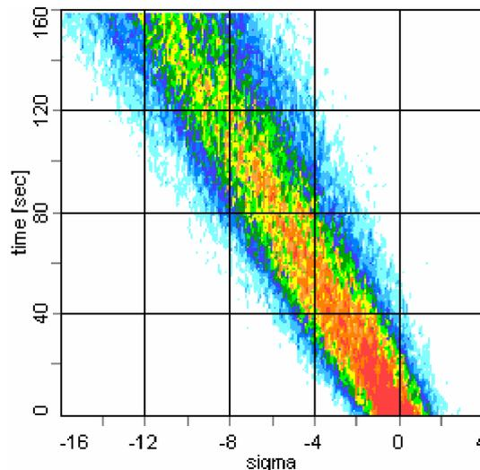
Fig. 1.2. Evolution of momentum spread distribution on time. The momentum is measured in initial rms width (sigma). The initial rms width is equal to  $2 \cdot 10^{-4}$ .
