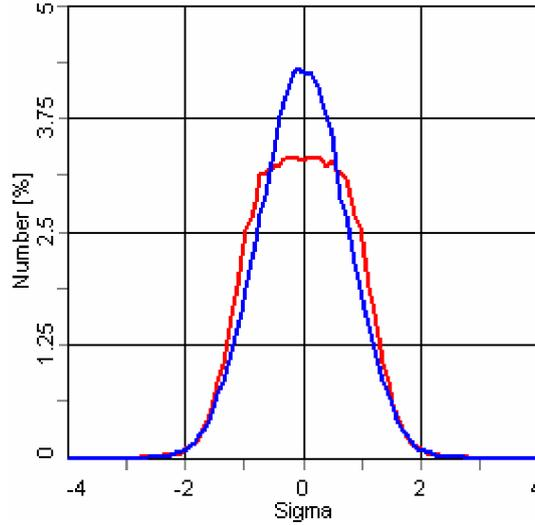
Fig. 3.2. Horizontal (red curve) and vertical (blue curve) beam profiles after 150 seconds of experiment. Initial effective target thickness is  $1.3 \cdot 10^{16}$  Atoms/cm<sup>2</sup>.
