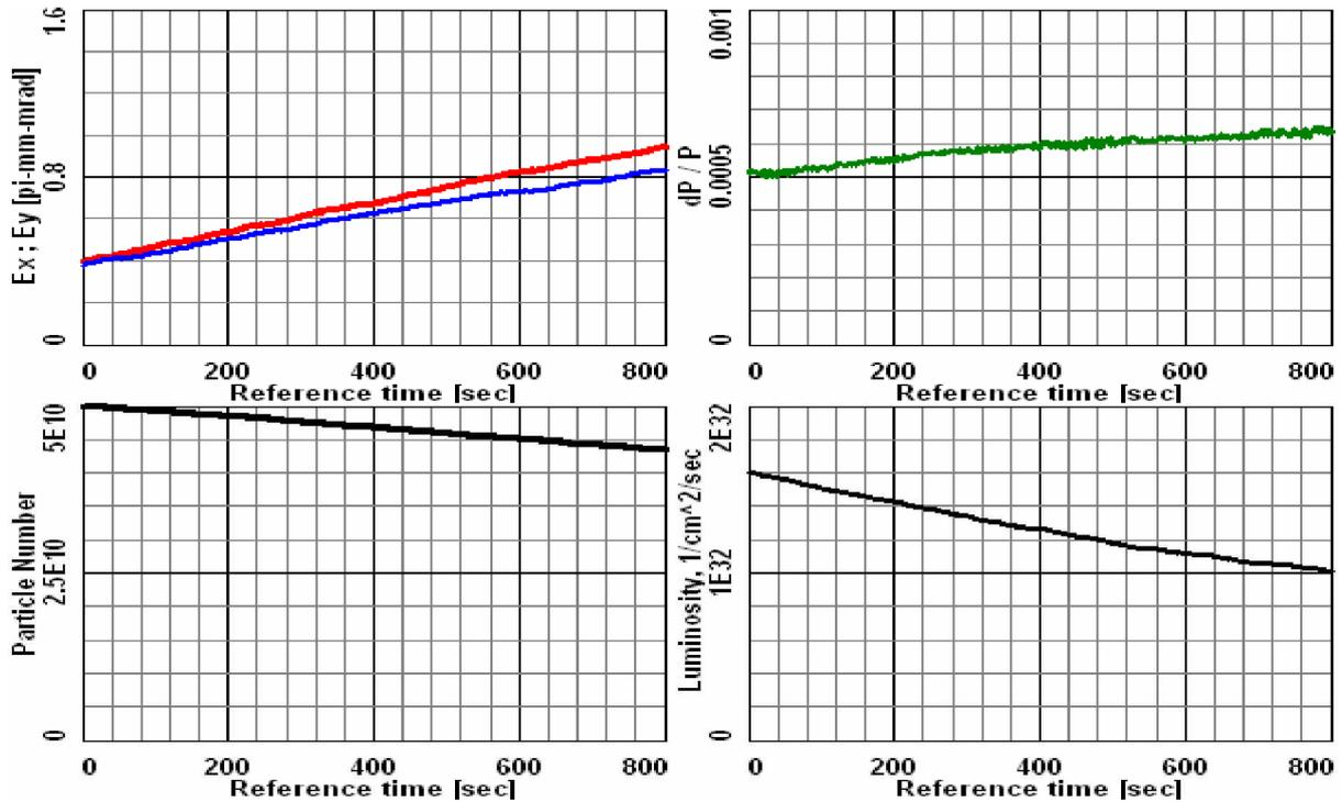
Fig.2.2. Evolution of beam parameter without cooling. Proton momentum is 3.7 GeV/c
