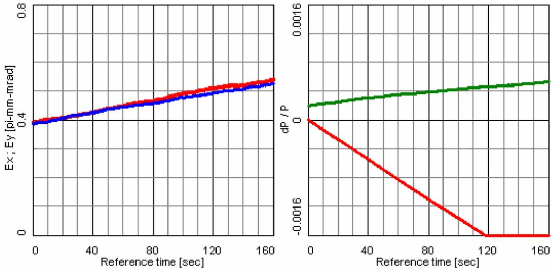
Fig.1.1. Emittance (left plot) and momentum spread (right plot) evolution in time due to interaction with internal target. The target density is  $2 \cdot 10^{15}$  Atoms/cm<sup>2</sup>. Grin line in the right plot is the relative momentum spread, red line – relative momentum deviation from its initial value.
