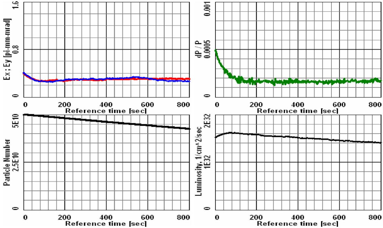
Fig.2.13. Evolution of beam parameter with electron cooling.
