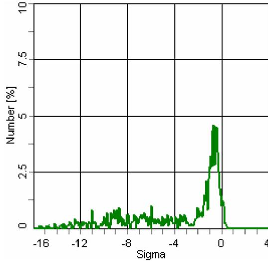
Fig. 1.4. Momentum spread distribution after 160 sec of interaction with internal target and electron cooling. Parameters are the same as in Fig. 1.3.
