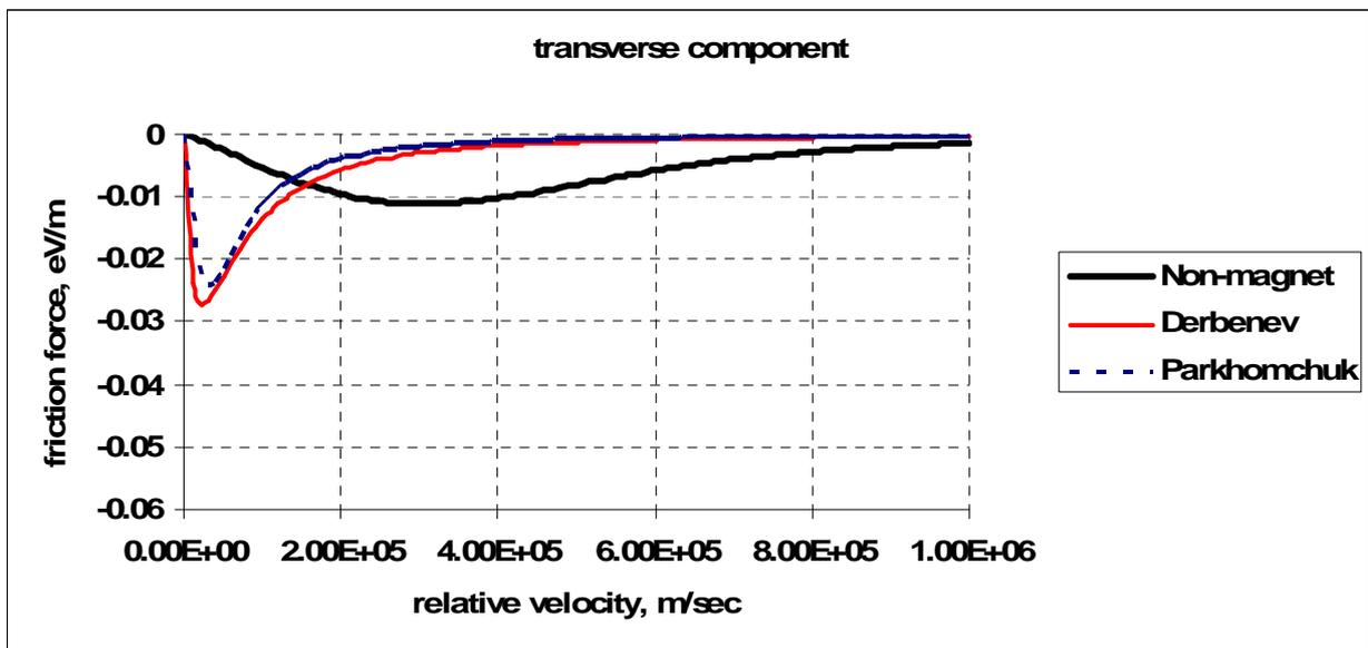
Fig.2.8. Ddependence of friction force components on the relative velocities between protons and electrons for different models of electron cooling ( $I_e=0.4A$ ).
