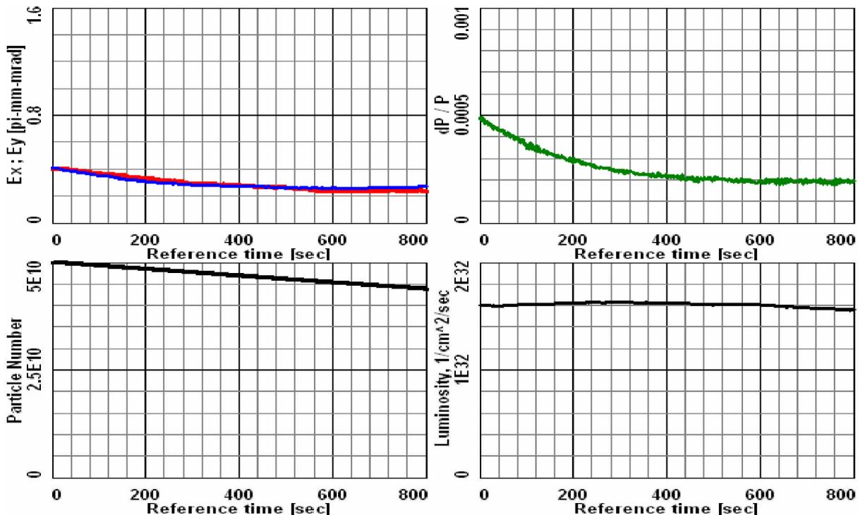
Fig.2.12. Evolution of beam parameter with electron cooling.
