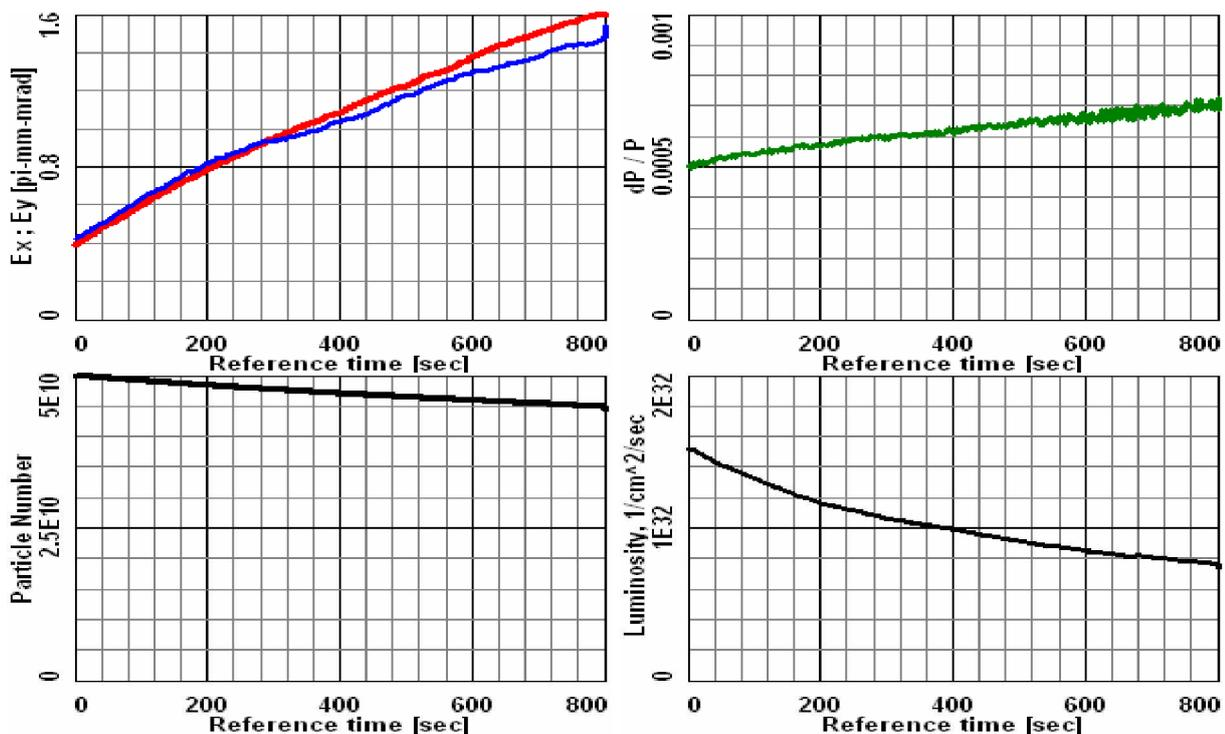
Fig.2.3. Evolution of beam parameter without cooling. Proton momentum is 2.25 GeV/c
