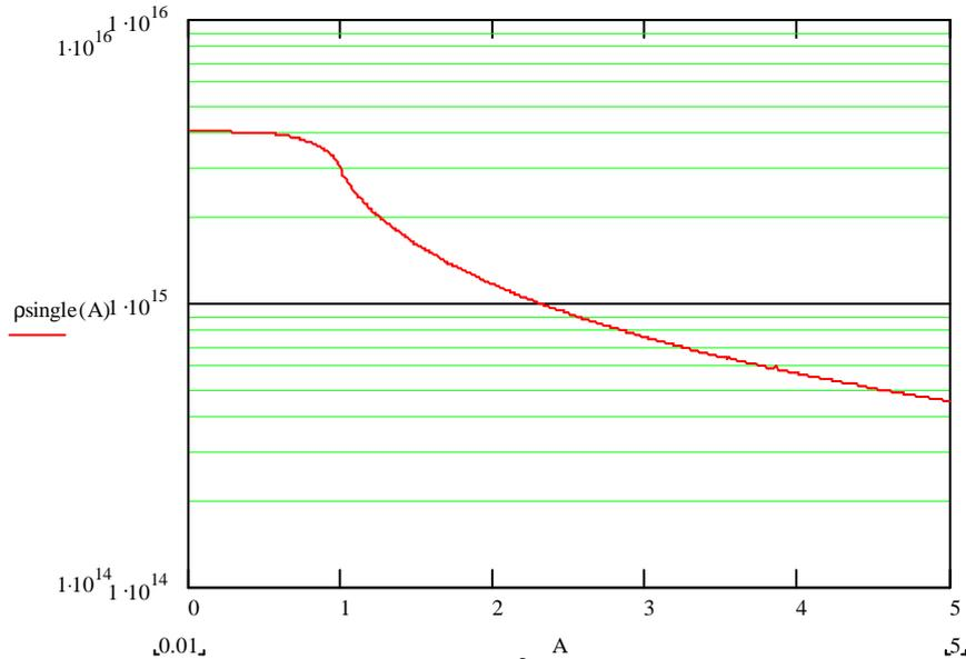
Fig. 1.7. Effective target thickness in Atoms/cm<sup>2</sup> versus amplitude of the particle horizontal betatron oscillations in mm. The flux radius is 1 mm. The target parameters are listed in the Table 2.1.
