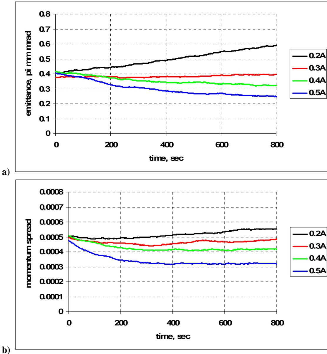
Fig.2.4. The dependence of emittance (a) and momentum spread (b) for coasting beam on time for different values of electron beam current (Parkhomchuk model).
