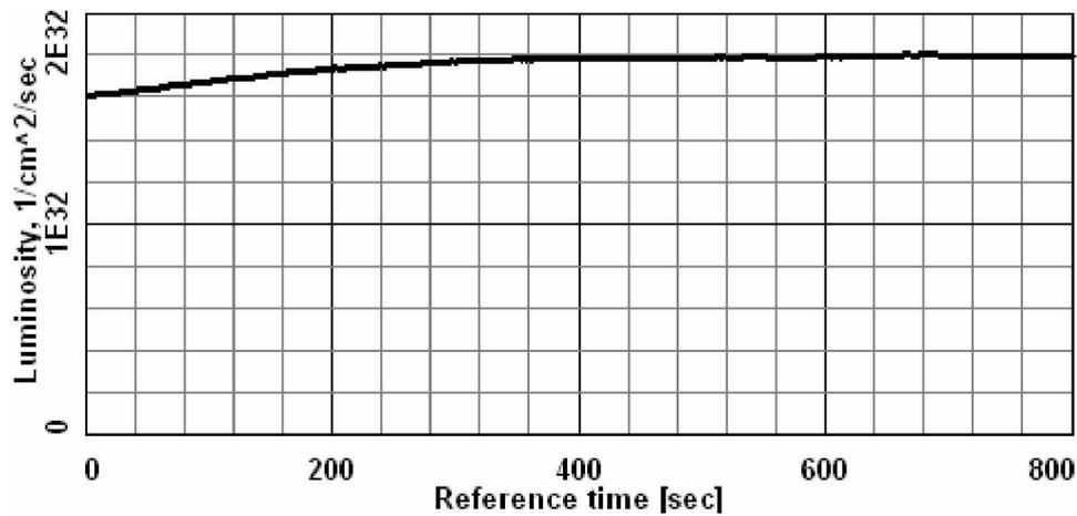
Fig.2.10. The dependence of luminosity for bunched beam on time at electron cooling ( $I_e=0.2\text{A}$ ).
