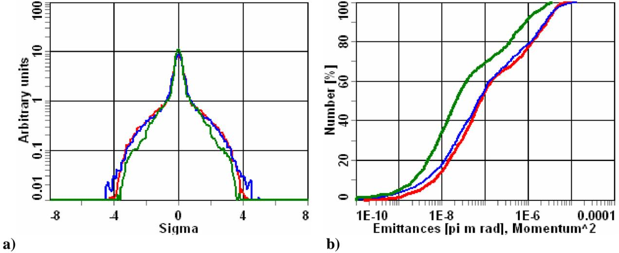
Fig.2.7. Transverse (a, red and blue) and longitudinal (a, green) profiles and distribution of invariants (b) of cooled bunched beam ( $I_e = 0.4$  A).
