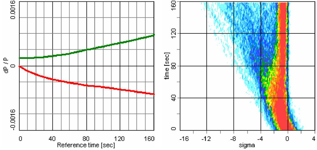
Fig.1.3. Momentum spread (green line in the left plot), momentum deviation (red line in the left plot) and momentum spread evolution (right plot) on time during interaction with internal target and electron cooling. Initial rms momentum spread is equal to  $2 \cdot 10^{-4}$ , the target density is  $2 \cdot 10^{15}$  Atoms/cm<sup>2</sup>, electron beam current is 3 A.
