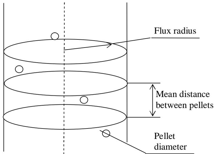
Fig. 1.5. Schematics of the pellet target geometry. The pellets move in the vertical direction from top to bottom with equal velocities.
