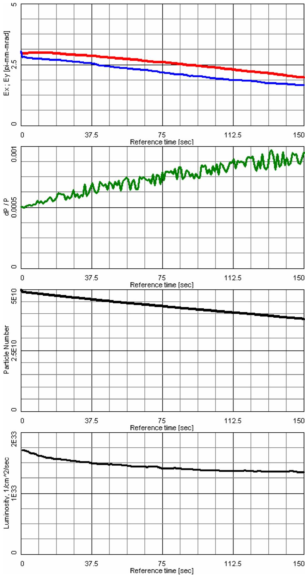
Fig. 3.1. From top to bottom: evolution of the beam emittance, momentum spread, proton number and luminosity under the common action of internal target, intrabeam scattering and transverse stochastic cooling. Initial effective target thickness is  $1.3 \cdot 10^{16}$  Atoms/cm<sup>2</sup>.
