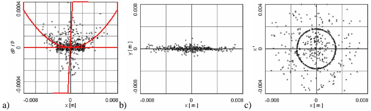
Fig.6. Distribution of model particle: momentum spread on horizontal coordinate (a), transverse profile (b), transverse phase space (c).  $N_p=3 \times 10^7$ ,  $I_e=100$  mA,  $M=2/0$  mrad (horizontal/vertical misalignment angle).
