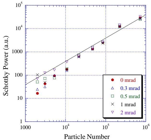
Fig.13 Schottky power as a function of particle number for different misalignment angles. The electron current is 25.5 mA at (a), (c), (d) and 102 mA at (b). The misalignment is the horizontal direction at (a), (b) and the vertical direction at (c) and both directions at (d). The solid line is  $P_{\text{Schottky}}=0.04 \times N_p$ .
