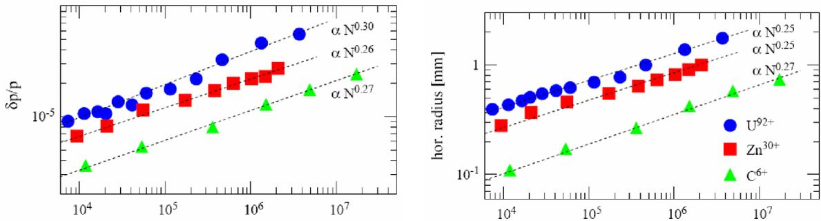
Fig.20. Dependence of momentum spread and horizontal size on particle number, measured at ESR.
