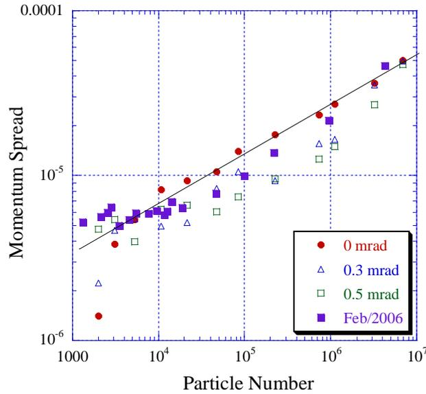
Fig.14. Comparison with the data in February, 2006 and the data with the misalignment in the both directions, which was subtracted from Fig.2 (d).
