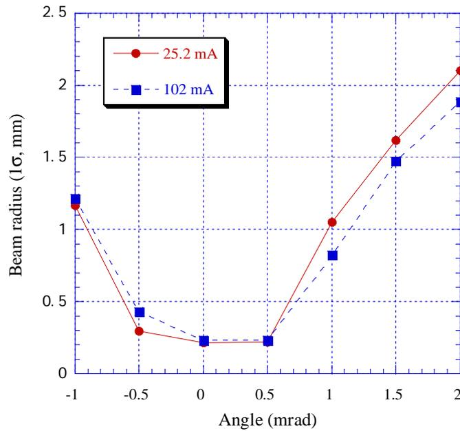
Fig.8. Transverse beam radius as a function of the misalignment angles, measured at two different electron currents. The particle number was  $1 \times 10^7$  (25.2 mA) and  $3 \times 10^7$  (102 mA)
