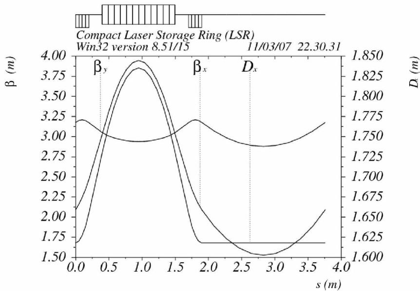
Fig.2. The lattice parameters of one period.
