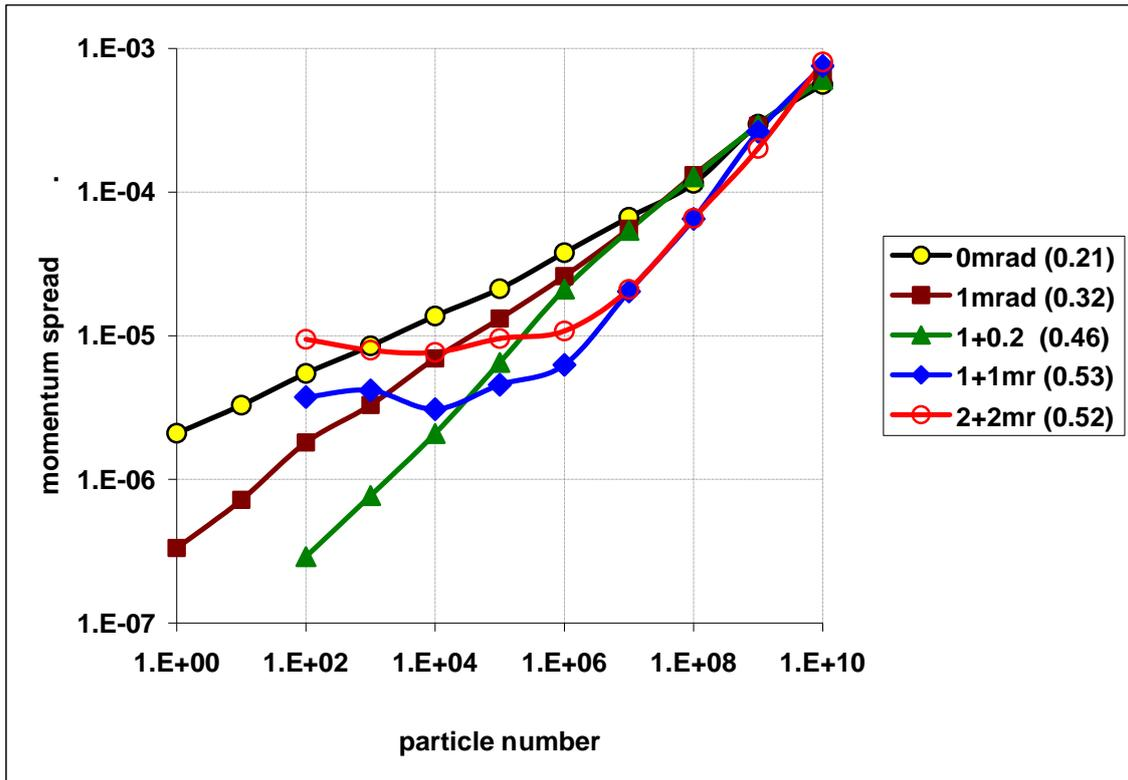
Fig.16. The dependence of the momentum spread on the particle number for different misalignments.  $I_e=25$  mA,  $M=0/0$ , 1/0, 1/0.2, 1/1 mrad,  $\xi=0.21$ , 0.32, 0.46, 0.53, 0.52.
