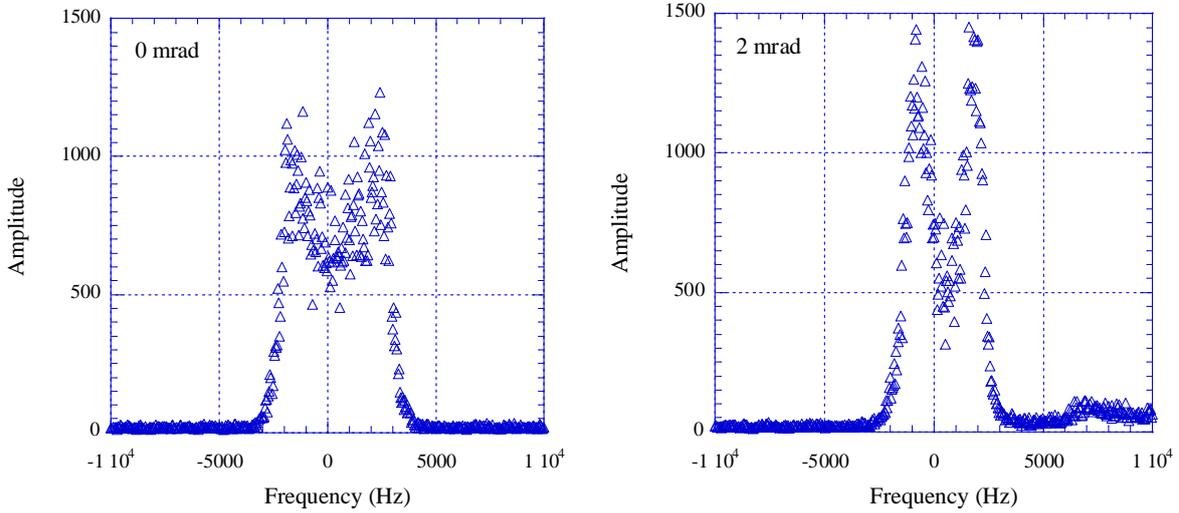
Fig.4. Schottky spectrums with the particle number of  $3 \times 10^7$  and the electron current of 102 mA. The misalignment angles are 0 and +2 mrad.
