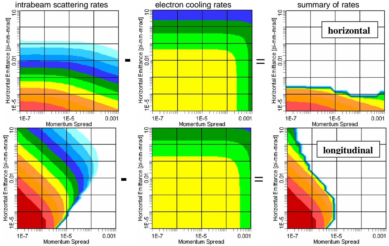
Fig.18. Intrabeam scattering rates (Martini model,  $N_p=10^3$ ) and electron cooling rates (Parkhomchuk model,  $I_e=25$  mA) for the S-LSR lattice structure. Each color corresponds to certain level of heating / cooling rates [1/sec], rate values are shown in Fig.19.
