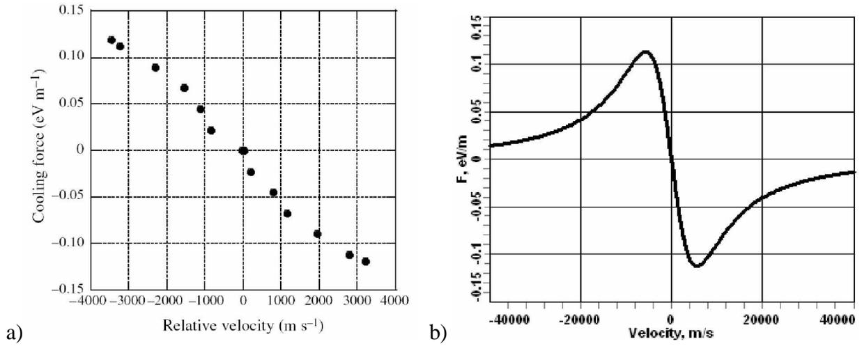
Fig.10. Measured longitudinal cooling force at an electron current of 50mA and ion current of  $0.1 \mu\text{A}$  using an induction accelerator (a), simulation results of the cooling force (b) for  $I_e=50 \text{ mA}$ ,  $T_{\perp}/T_{\parallel}=34/0.02 \text{ meV}$ .
