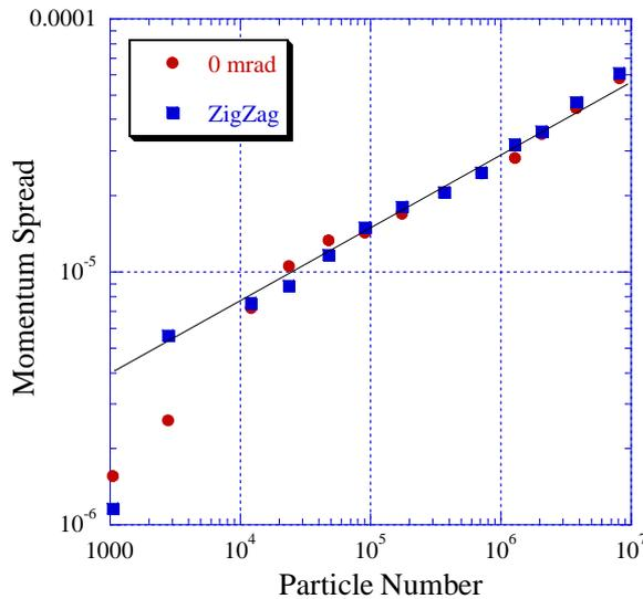
Fig.15. Measured momentum spread of a stored proton beam as a function of proton number. The blue marker corresponds to the normal field, and in the measurement described by the red markers a zigzag field, created by the vertical correction coils, was used.
