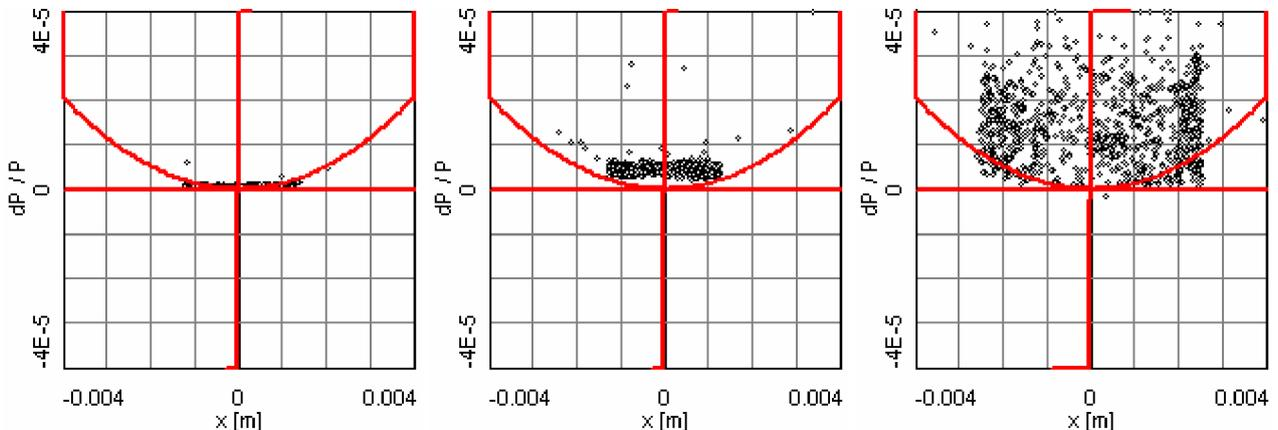
Fig.17. The particle distribution in the cooler section, points – model particles, red parabola describes the space charge parabola of the electron beam.  $I_e=25$  mA,  $N_p=100$ ,  $M=1/0.2$ , 1/1, 2/2 mrad.
