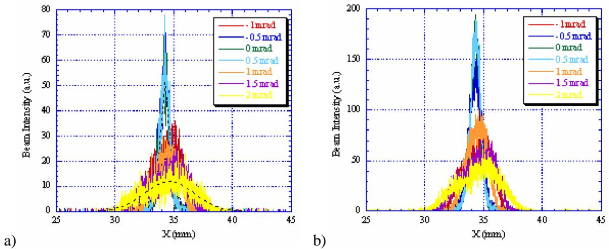
Fig.7. Transverse beam profiles measured by the ionization monitors. The electron current was 25.5 mA (a) and 102 mA (b). Horizontal misalignment angles  $M=-1, -0.5, 0, 0.5, 1, 1.5, 2$  mrad.
