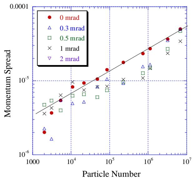
Fig.12 Momentum spread as a function of particle number for different misalignment angles. The electron current is 25.5 mA at (a), (c), (d) and 102 mA at (b). In (a), (b) a horizontal misalignment, in (c) a vertical and in (d) in both direction was chosen.
