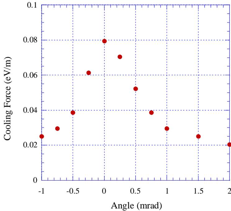
Fig.11. Maximum longitudinal cooling forces measured for different horizontal misalignment angles, using the induction accelerator. The electron current was 25.5 mA.
