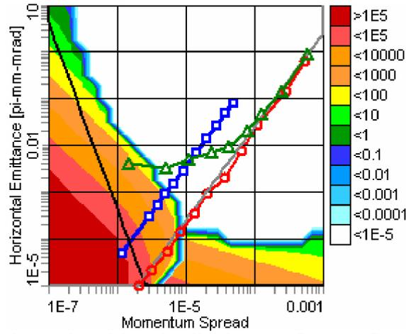
Fig.19. Overlap of horizontal and longitudinal sum of rates. **Gray line** –equilibrium of transverse and longitudinal temperature of proton beam, **black line** –  $\Gamma_2$  ordering criterion [15], blue square ( ) – experiment (line without point means drops to ordered state), red points (O) – simulation with zero misalignment, green triangle ( $\Delta$ ) – simulation with 0.2/0.2 mrad misalignment.
