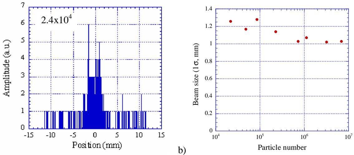
Fig.9. Transverse beam profile measured at a horizontal misalignment of 1 mrad (a) for  $N_p = 2.4 \times 10^4$  and transverse beam size as a function of the particle number (b).
