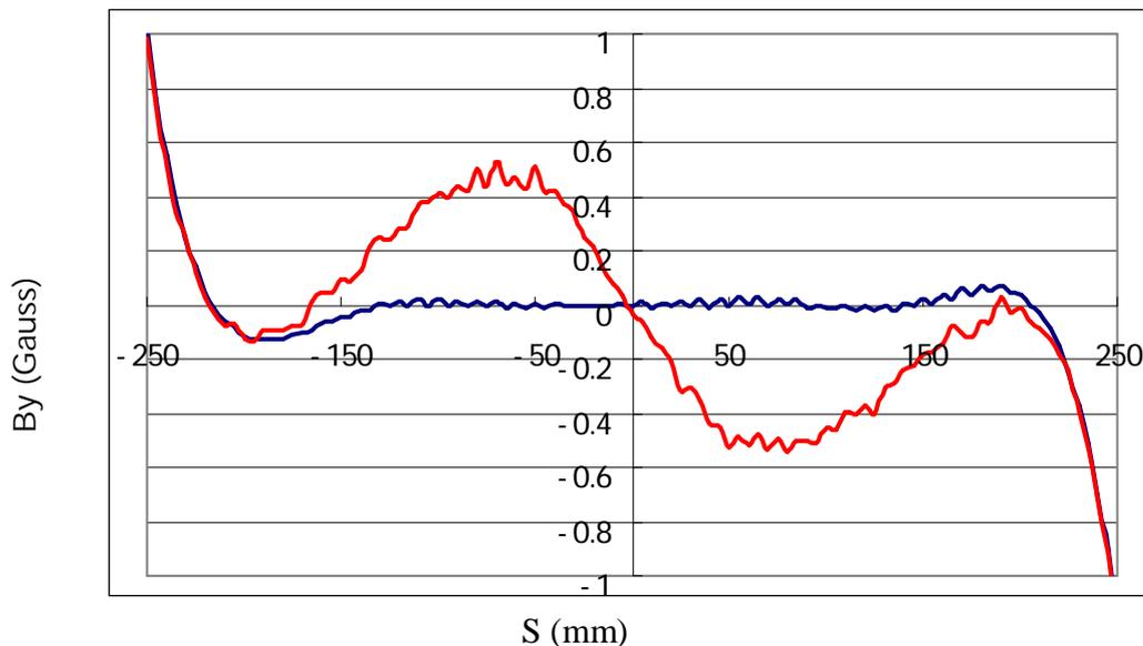
Fig.3. Vertical component of the magnetic field in the cooler solenoid coil. The blue line is the present field. The red line is the zigzag field created by the correction coils.
