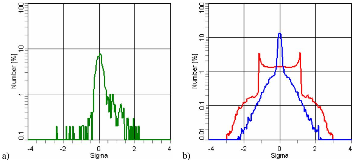
Fig.5. Simulation of momentum spread (a) and transverse profiles (b) for  $N_p=3 \times 10^7$ ,  $I_e=100\text{mA}$  and horizontal misalignment 2 mrad. Red line – horizontal profile, blue – vertical one.
